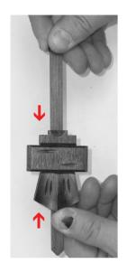
If the clock runs too fast, take off the pendulum and slightly move down the leaf/shield. Hang back in the pendulum and try the clock. If it still runs too fast, repeat the aforementioned.
