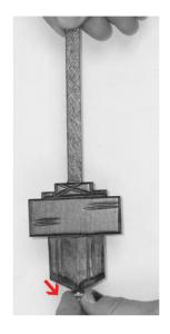
Some of our have a screw pendulum. The speed of the clock is regulated by the length of the pendulum. The pendulum length can be changed by turning the adjustment nut on the bottom of the pendulum.
