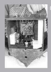
2. If you cannot easily close the door by hand, completely pull up the weights, take off the weights and pendulum, open the back lid (see "cuckoo clock manual" #2a) and check in the open back if the wire that is marked with a red (1) is underneath the cuckoo's tail. If not, please move it underneath the tail. Close the back lid, hang the clock back on the wall, and put all parts back on.
