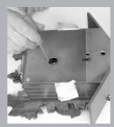
3. If the chime still makes a rattling sound, pull the chains completely up. Take off weights, pendulum and top part (only traditional carved cuckoo clocks). Take the clock from the wall. Put clock face down on a thick newspaper or cloth. On the lower side of the back lid you see a round hole. Behind the hole you see part of the gold plaited chime wire. Take a screwdriver, put it in the hole and slightly bend down the chime wire.
