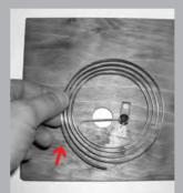
2. Check if the chime touches the back wall. Open the back lid (see #I above). Put the back lid on a table in an upright position. If the chime wire touches the back wall, take the wire and slightly pull it opposite from the wall until it slightly bends and does not touch the wall anymore.
